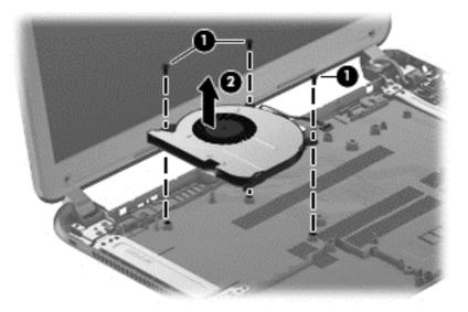
Reverse this procedure to install the cooling fan in the base enclosure.
